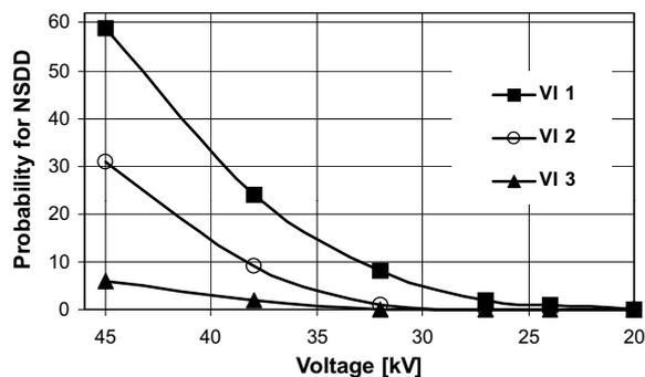
Figure 5: Probability of an opening operation with at least one NSDD as function of the applied voltage
