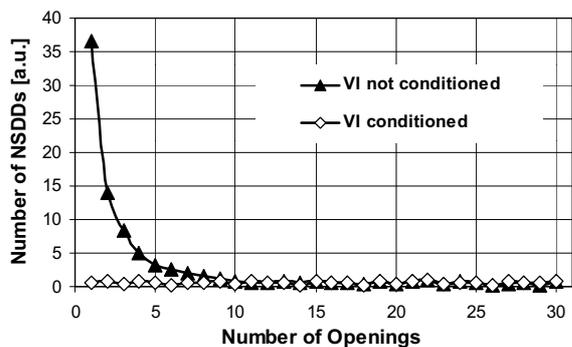
Figure 6: Number of NSDD depending on the number of subsequent openings both before and after conditioning at 45 kV
