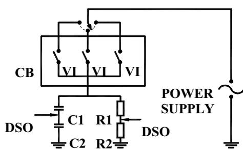
Figure 2: Electrical circuit used for NSDD investigation
