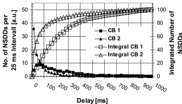
Figure 3: Time dependence of NSDD for two different circuit breaker types
