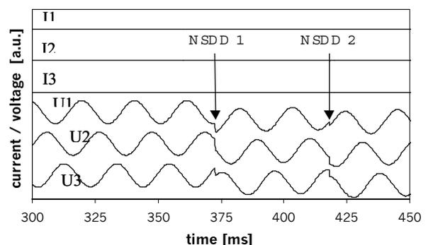
Figure 1: Typical Non-Sustained Disruptive Discharges in a three-phase circuit
