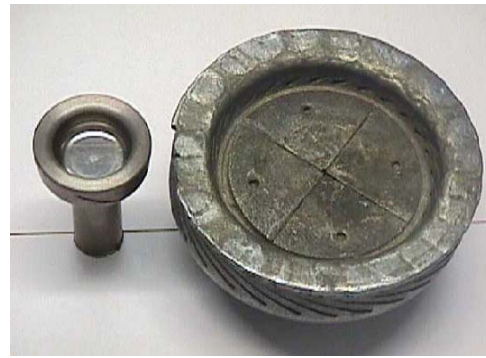
Fig. 9 Comparison of size of contact for 12kV 20kA rating.
