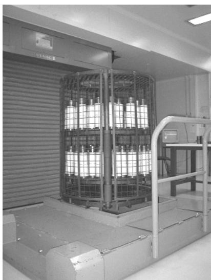
Figure 6 ; Interrupters assembled ready for One Shot Seal Off process in Vacuum Furnace
