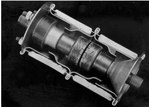
Figure 2. V8 12-25 interrupter, c.1981 using Contrate contact, Glass-Ceramic insulators, and a brazed-welded-furnace seal off manufacturing system.
