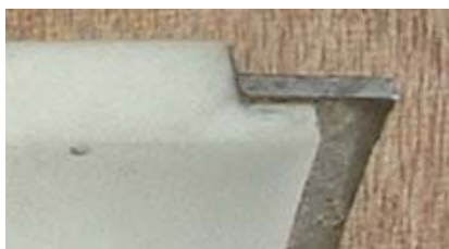
Figure 8. Actual shielded braze joint
