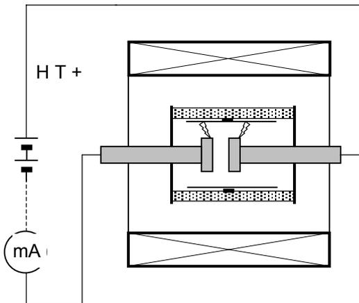
Figure 3: Vacuum interrupter in Magnetron coil connected for Double Inverse Magnetron mode.
