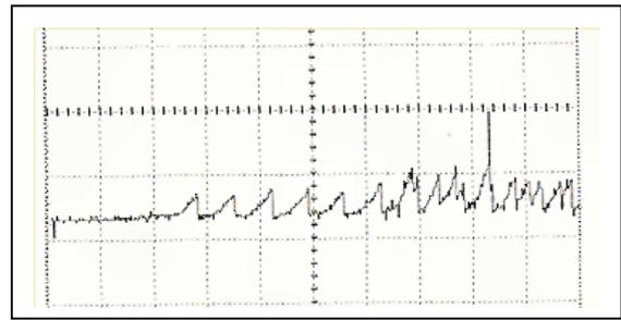
Fig. 7: SIM waveform at 1kV. The current scale and the timebase are expanded by 10x compared to those in Fig. 6.
