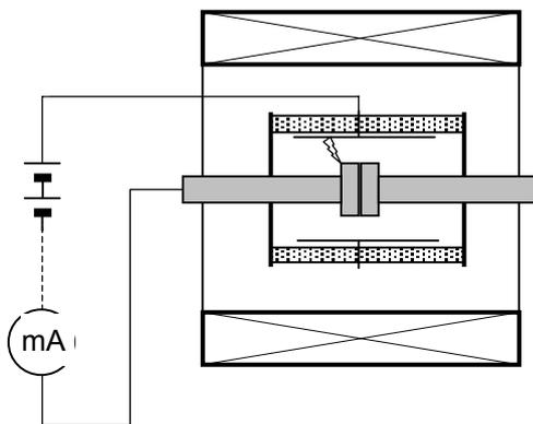
Fig. 1: Vacuum interrupter in Magnetron coil connected for Single Inverse Magnetron mode.
