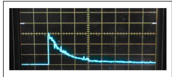
Fig. 2: Typical current pulse for a single inverse magnetron discharge.
