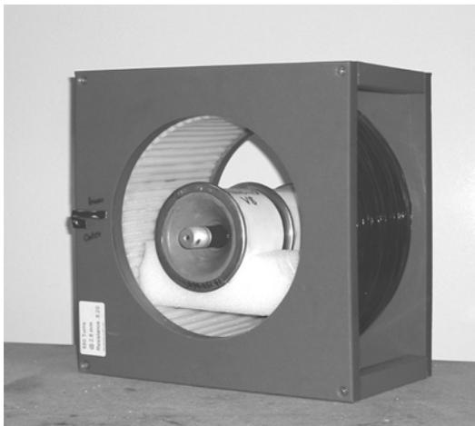
Figure 4: A vacuum interrupter in position in the solenoid coil.
