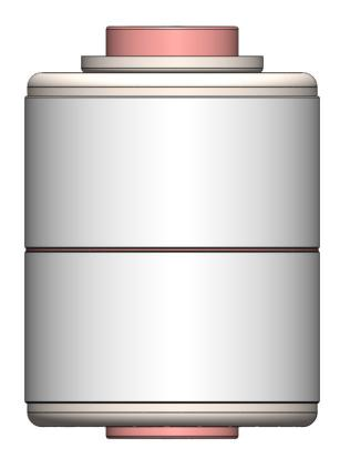
This is a concept Vacuum Interrupter with a special arc control device which can interrupt DC of 31.5kA at Medium voltages (12kV). It is a concept at present, and will be tested early next year. If successful then scaling up to 30kV and beyond should be possible.
