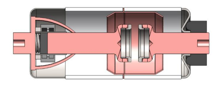
This is a "SAVI" Vacuum Interrupter with a combined Rogowsi Coil and Voltage Sensor fitted to the conductor. It also has a vacuum measurement device fitted to allow present status and prediction of vacuum life to be assessed during the service life of the Interrupter
