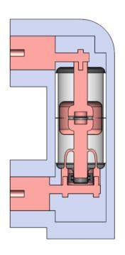
This is the same unit but with a SAVI Vacuum Interrupter fitted.
