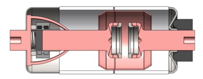
This is a "SAVI" Vacuum Interrupter with an internal magnetic actuator built into the device. It does not require any external mechanism and has no bellows, or externa Imoving parts. This means that, for example it can be completely encapsulated without difficulty
