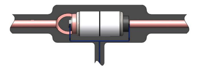
This is a "SAVI" Vacuum Interrupter which is mounted as a cable joint.
